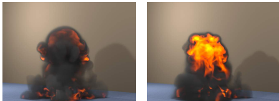
Figure 7: Smoke plumes which result from a detonation within an enclosed chamber (left), and from a detonation within a chamber whose front left wall is fragile (right).
